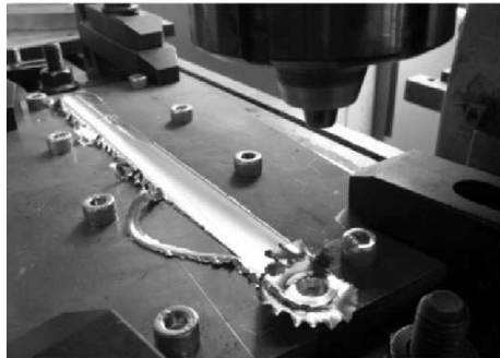
Fig. 1. Experimental setup used for the diagonal friction stir weld, (a) photograph of weld D2 and (b) scheme
